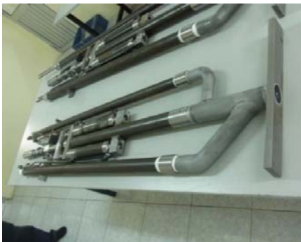
Grout Injection Pipe overall view
